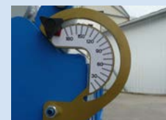
Angle limit stop 0-155° (Available only for the TRIADÉ OPIUM®)
