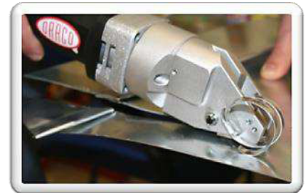
cutting through double lock seam 6 times folded at the ridge or gutter
